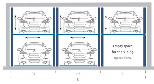
On the entrance level are sliding platforms with one empty space on the right (on the left: possible as an option). On the upper level the system is provided with lifting/lowering platforms.
