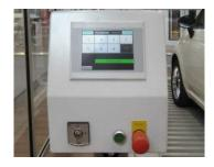
Touch screen with key switch, emergencystop in dead man's control with brief operating instructions fastened on the wall and cabling to the power unit.
