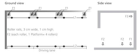
L1 and L2= Distance of the rails from the back wall (in cm). (L1= 105, L2= 477)
