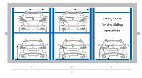
On the entrance level are sliding platforms with one empty space on the right (on the left: possible as an option). On the lower level the system is provided with lifting platforms. A lifting platform will be lifted to the empty space on the entrance level.
